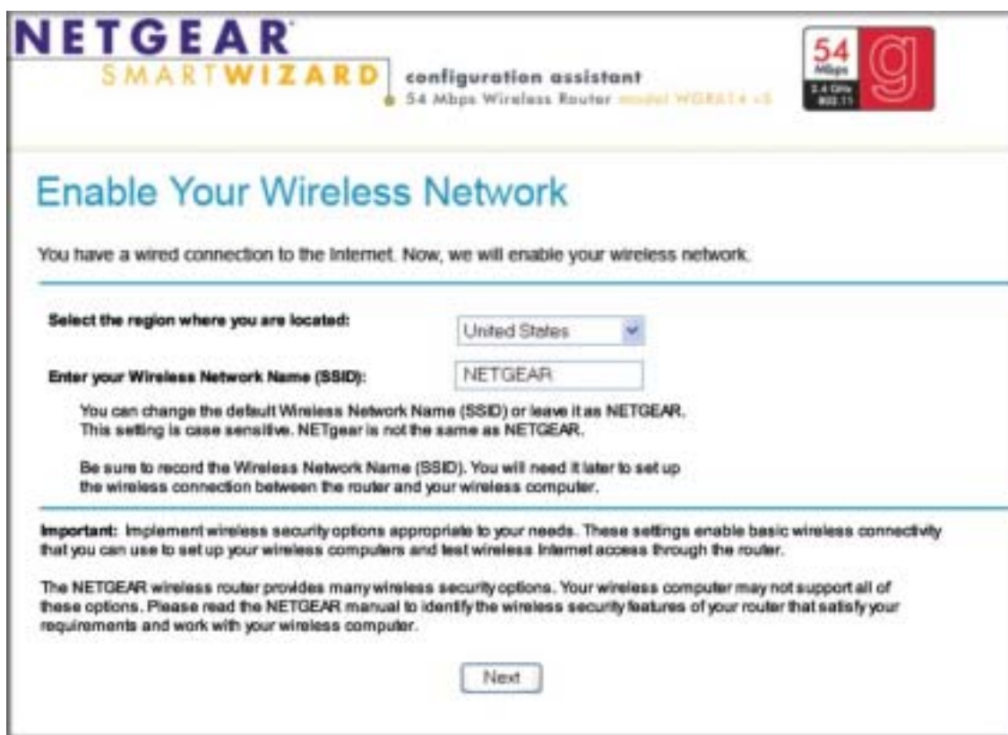
Figure 3-6: Enable the wireless feature
